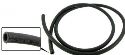
Breather hose with a textile outside per meter Inner diameter: 12mm, Outer diameter: 17mm, Working pressure: 7 bar, Bursting pressure: 30 bar
