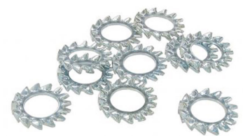
External serrated lock washers M8 (10 pieces) Inner diameter: 8,4mm, Outer diameter: 15mm, Height: 2.4mm, Material: Galvanized steel
