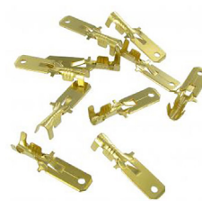
Uninsulated male spade connectors with locking barb (10 pieces) Spade connector size: 6.3mm, Material thickness: 0.8mm, Wire thickness: 1.5 - 2.5mm 2
