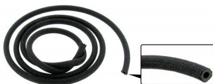
Vacuum hose with a textile outside per meter Inner diameter: 3.5mm, Outer diameter: 7.5mm, Working pressure: 7 bar, Bursting pressure: 30 bar
