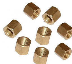
Brass nuts (8 pieces) Thread size: M8 X 1.25, Wrench size: 11mm
