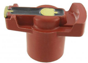
Rotor (5 kilo-ohm) Type-1 engines 30hp 8.1959 and later, 34hp until 7.1965, 1200, 1300, 1500 and 1600cc 8.1968 and later, Type-3 engines 1500cc 8.1968 and later, 1600cc 8.1968 until 7.1969, Type-4 engines Bus until 7.1979, Waterboxer engines 1900cc, 009 distributors
